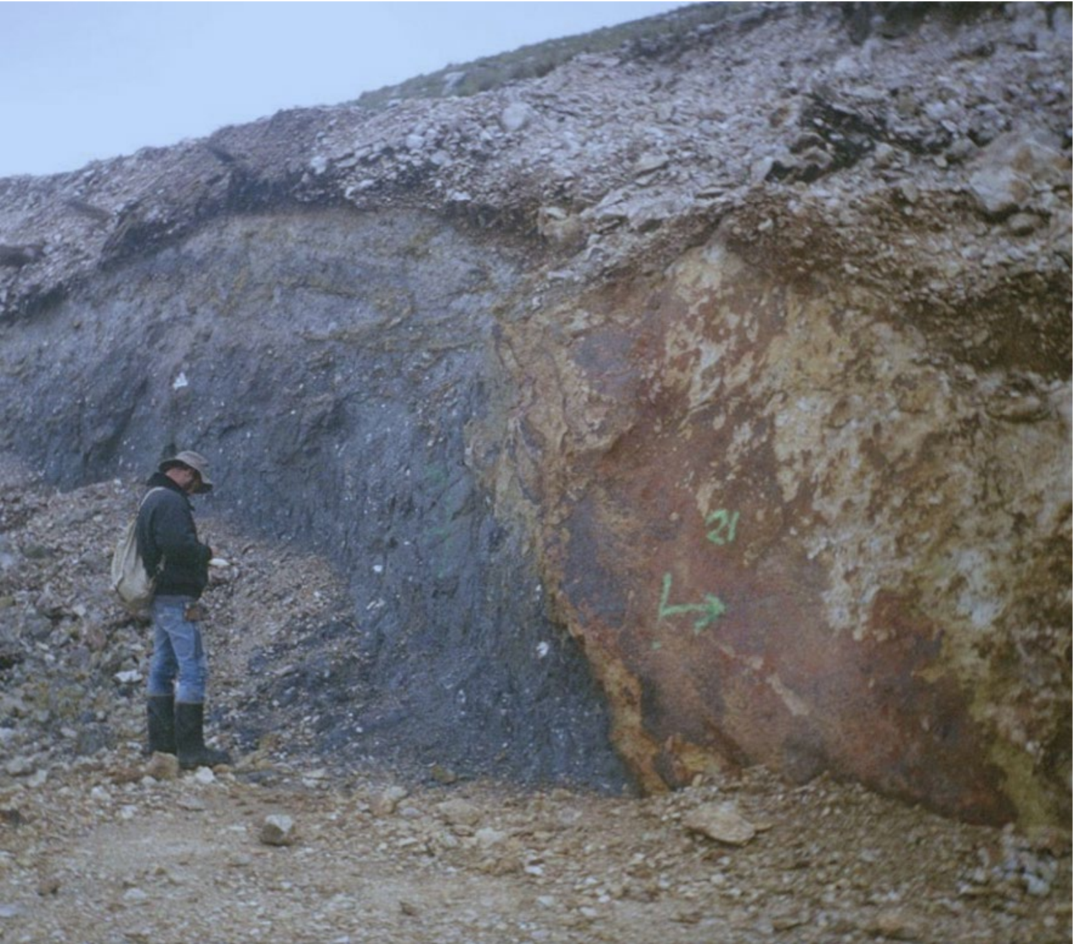
Oxide mineralization in andesite with a pre-mineral rhyolite caprock
