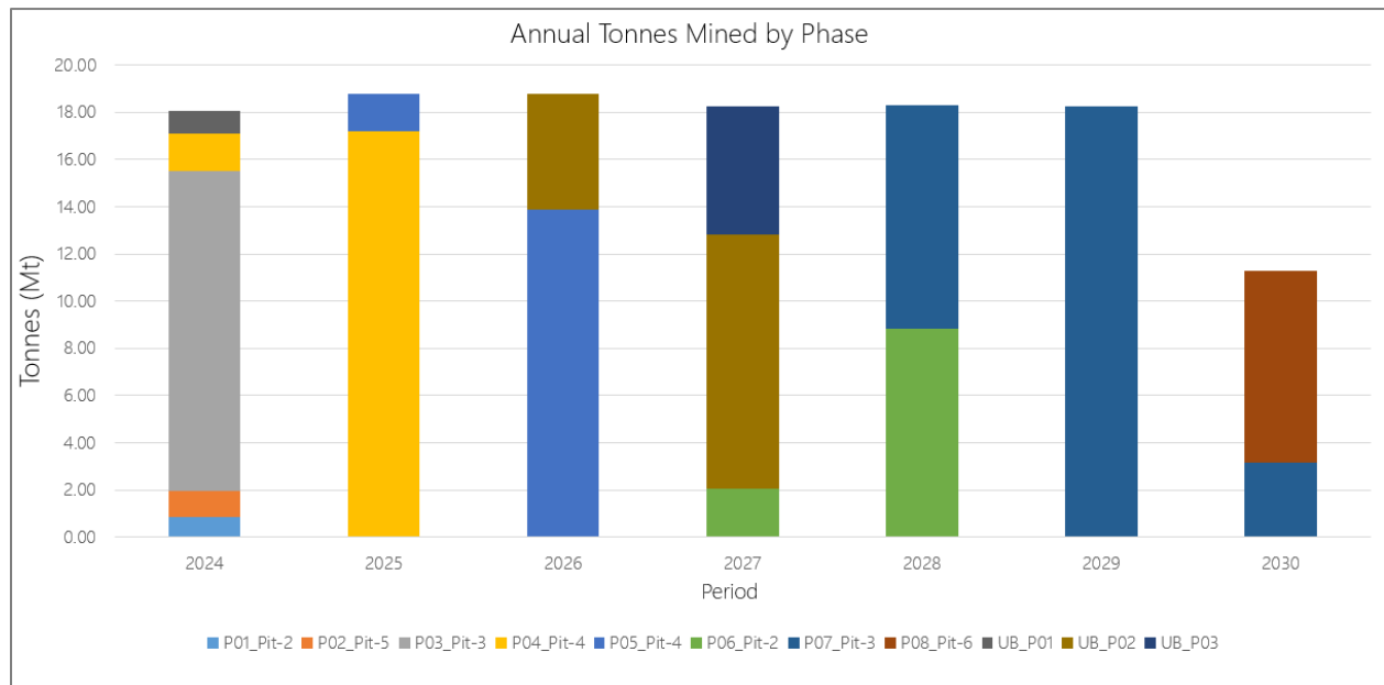
Figure 16-4: Annual Tonnes Mined over the Boroo and Ulaanbulag Life of Mine by Phase
