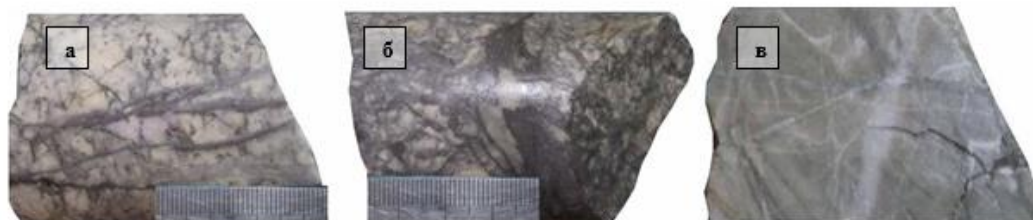
a, b-granite with sericite-silicified transformation, c-quartz-sericitized diorite
